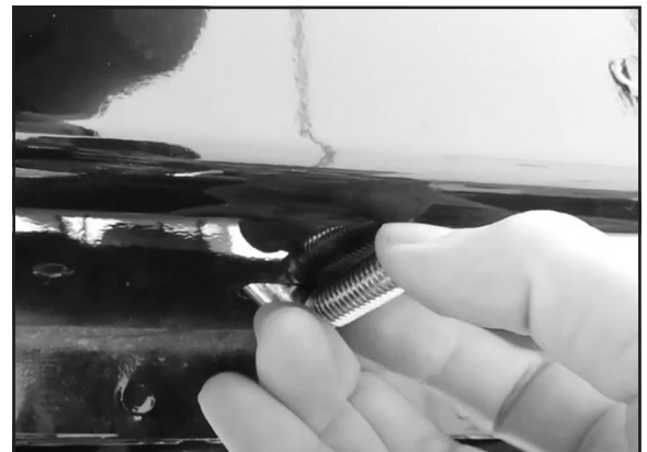
(Figure 5) Insert the bend on the tail into the slot, keeping the threads pointed outwards.
