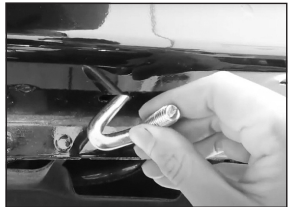
(Figure 4) Insert the tail on the Spiral Bolt into the slot, keeping the threads pointed outwards.
