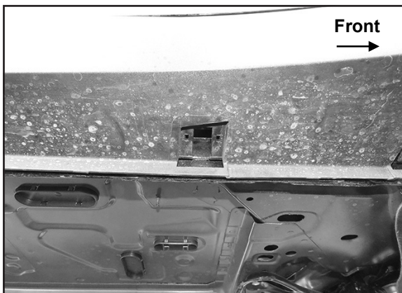
(Figure 2) Passenger/right #2 clip removed.
