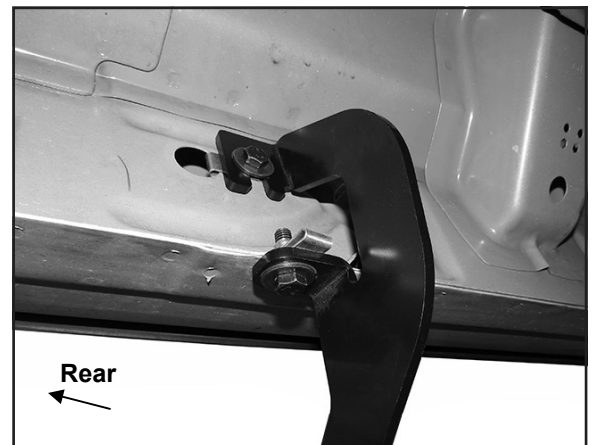
(Figure 8) Example of driver/left rear Bracket attached to location with 8mm Clip Nuts.
