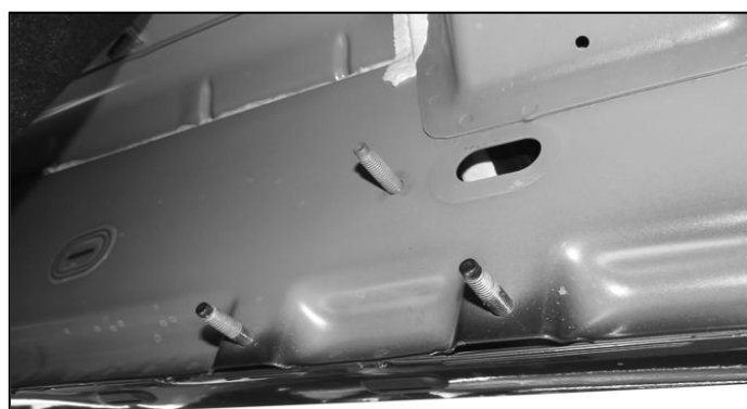
(Fig 4) Attach (1) Mounting Bracket to the front mounting location
