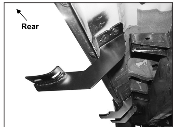
(Figure 6) Driver/left rear Mounting Bracket installed.
