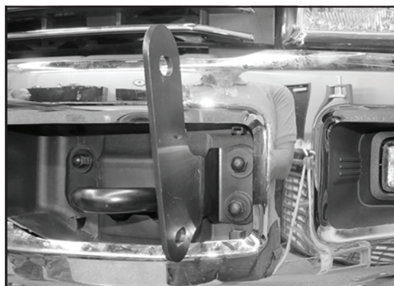
(Figure 4) Reuse factory bumper bolts to attach driver/left Frame Bracket to bumper.
