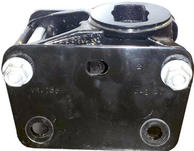
OEM side plate with "puck" installed & removed from truck frame
