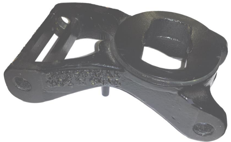
OEM "puck" removed from truck frame & OEM side plate
