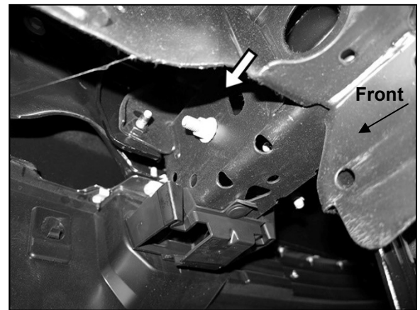
(Fig 15) 2022-on model, remove driver/left tow hook (pictured from behind bumper)
