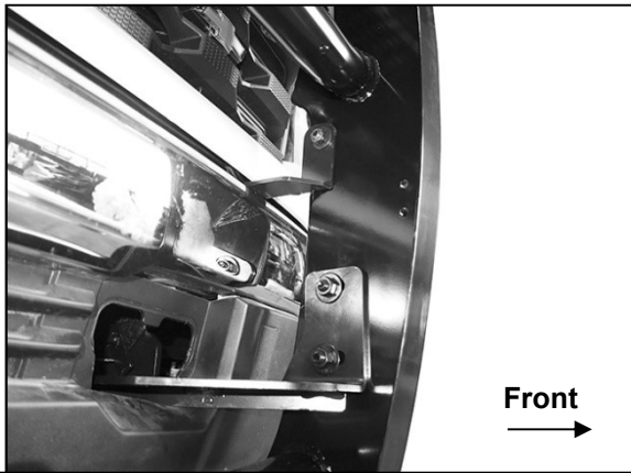
(Fig 43) Attach Grille Guard to driver/left side Brackets. 2022-on model pictured
