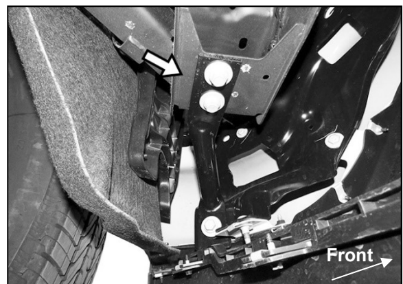
(Fig 31) 2022-on model bumper removal for tow hook reinstallation. Remove outer bumper supports (arrow). Driver/left side pictured.
