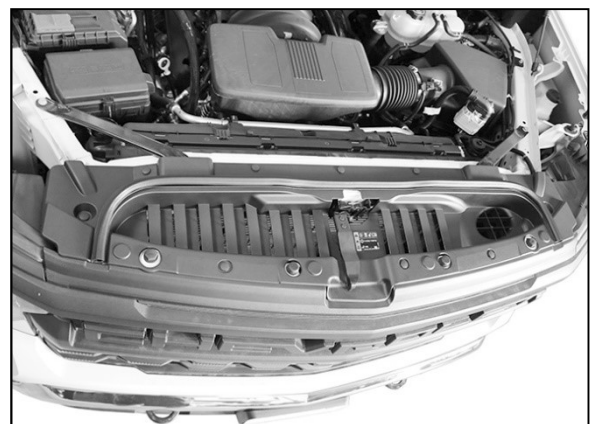
(Fig 19) 2022-on model remove hood release lever and cover, (arrow). Also remove grille
