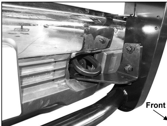
(Fig 40) Attach Grille Guard to Frame Brackets. Model with relocated tow hook pictured
