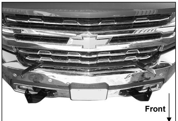
(Fig 13) 2019-21 model Brackets installed
