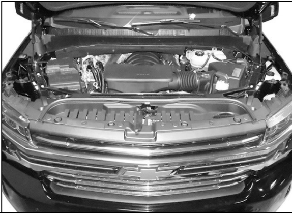
(Fig 8) Remove hood release lever and plastic cover from top of grille
