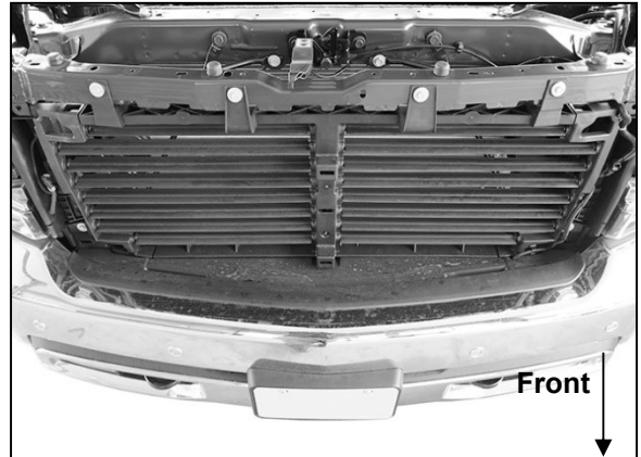
(Fig 9) Remove screws attaching grille and carefully pull grille straight out to remove
