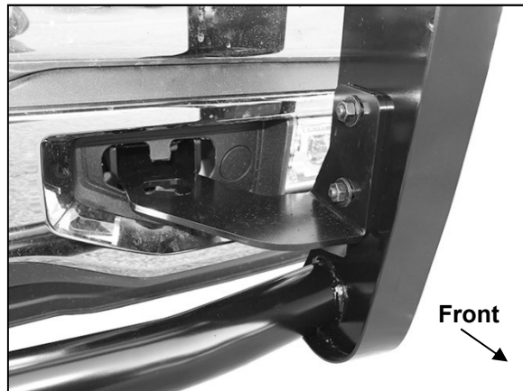
(Fig 39) Attach Grille Guard to Frame Brackets. Model without tow hook pictured
