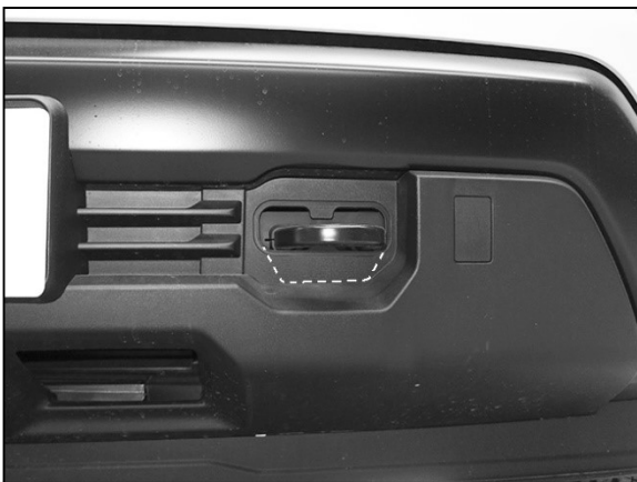
(Fig 16) 2022-on model, cut opening to clear Frame Bracket. Note dashed line for example only
