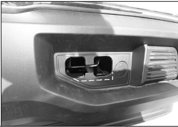
(Fig 3) Tow hook removed. Opening may need to be trimmed to clear the Mounting Bracket
