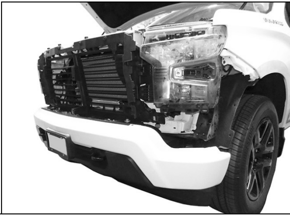
(Fig 20) 2022-on model, remove fascia body panel from top of bumper and remove grille
