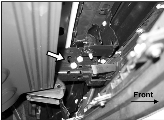
(Fig 14) 2022-on model, remove driver/left tow hook (pictured from behind bumper)
