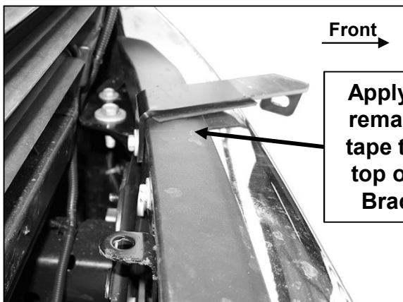
(Fig 12) 2019-21 Model, reuse factory hex bolt to attach Support Bracket to back of bumper
