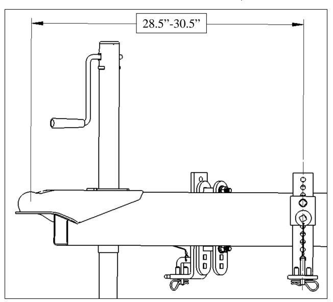
**Note:** When installing new frame brackets, set the position and height of the lift brackets to be the same as the previous ones so as to not change the setup of your "system"
