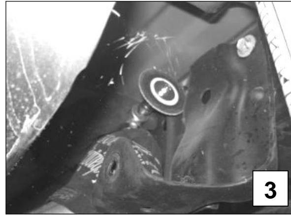
3b) Remove the rivet heads with a pneumatic hammer and chisel attachment. (**Photo 4**). It should take no more than a few seconds to chisel each head off. Once all rivet heads have been removed, it is helpful to use a punch and hammer or a punch with the air hammer to push out the remaining portion of the rivets.
