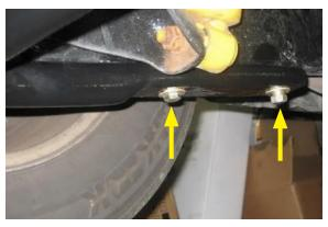
8. With the bolt holes at the ends of the sway bar facing up, position the new Belltech sway bar at the bottom of the lower control arms
