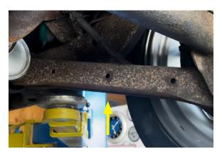
9. Fasten the Belltech sway bar to the control arms with the original bolts. Torque to 30 ft lbs.
