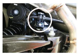
9. Detach the end links from the sway bar. Carefully guide the original sway bar through and above the exhaust system to detach the sway bar from the vehicle. If clearance is limited, remove the original bushings and brackets for additional clearance.
