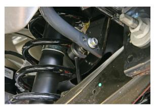
16. Torque the pivot bushing brackets to 16 ft lbs.
