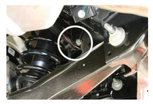
8. Remove the four 13mm bushing brackets bolts. Rest the sway bar on top of the exhaust for now.
