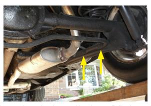
8. With the bolt holes at the ends of the sway bar pointed up, position the new Belltech sway bar inside the cavities of the lower control arms.
