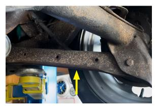
9. Place the supplied 7/8" spacers inside the control arms. Position them in line with the bolt holes on the control arm and the sway bar. Fasten the sway bar to the control arms with the 3/8" bolts and Nyloc nuts. Use the 3/8" washers at the bolt head and nut. Torque to 23 ft lbs.
