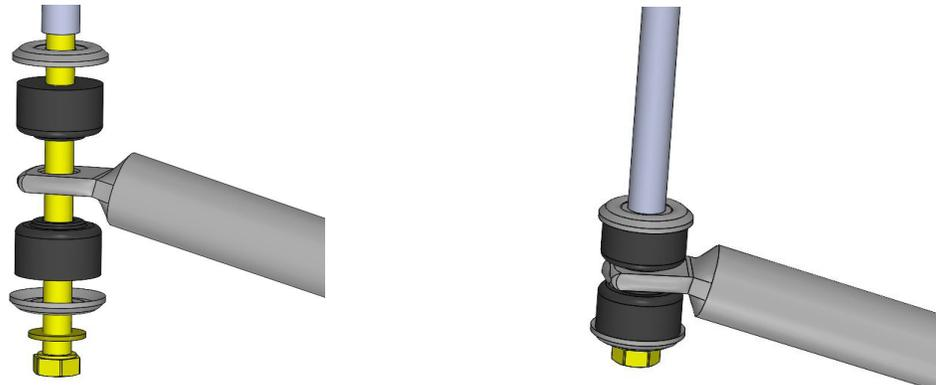
15. Mount the end link assembly to the chassis mount and tighten the end link bolt to the point where the spacer tube can still be forced to rotate on the bolt by hand, but the rubber grommets should not be able to rotate by hand.
