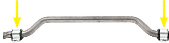
11. Ensure there is 1/32" to 1/16" of the bushing is showing after the bracket is seated. If the bushing is showing more than 1/16", use a sander or a sheet of coarse grit sandpaper to shave it down to the proper height.
