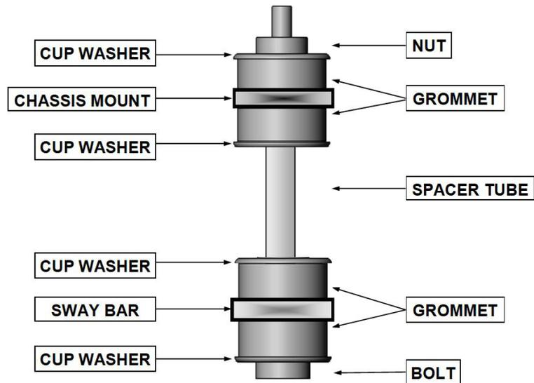
14. Assemble the end links to the Belltech sway bar, as shown in the diagram.
