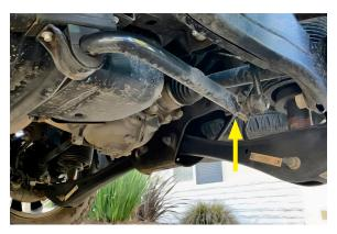
8. Remove the 10mm bolts from the pivot bushing brackets and detach the sway bar from the vehicle.
