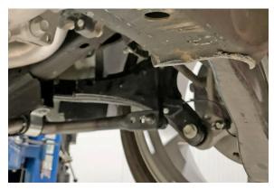
14. Adjust the position of the sway bar so it is centered from left to right and front to back. Torque the pivot bushing bracket bolts to 37 ft lbs.
