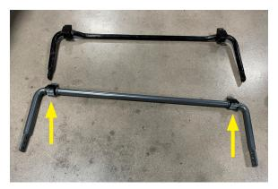
11. Place the Belltech sway bar and the bushing support plate on the chassis mount. The support plate is placed between the chassis and bushing bracket. Align the holes in the bracket and support plate with the original mounting holes. Use the supplied 10mm-1.5 x 35mm bolts and 3/8" washers to fasten the sway bar. Do not torque the bolts yet.
