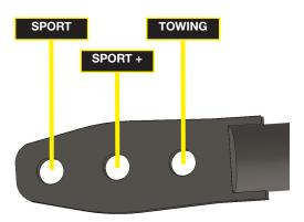
13. Attach the sway bar to the end links using the original nuts; torque to 74 ft lbs.
