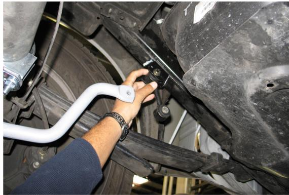
23. Use a floor jack to lift axle up to ride height, this will ease the fastening of the end links to the bar and the frame rail. Ensure not to lift the vehicle off the jack stands.
