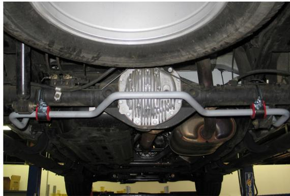
32. Torque the lower end link bolts to 40 ft lbs.
