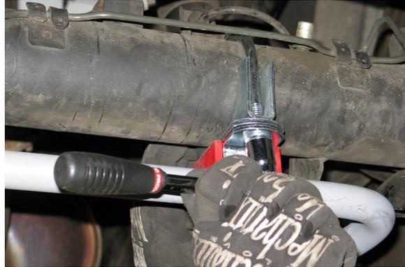
30. Center the sway bar left to the right and front to rear. Position the U-bolts and clamps to the widest spacing possible, within the lower shock mount brackets. This will prevent the sway bar from shifting left or right while cornering.
