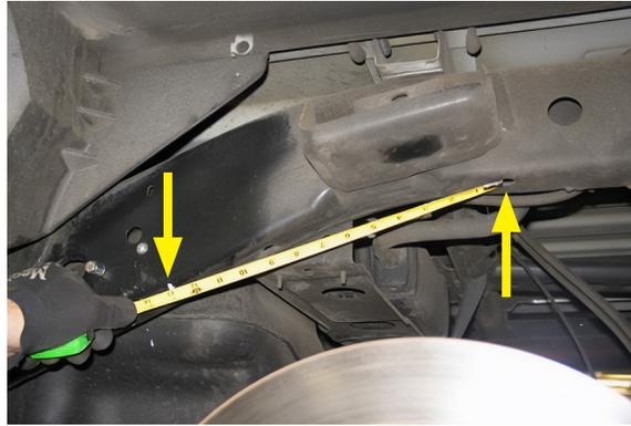
11. Use a marking pen to mark the edges of the bracket onto the frame as shown.
