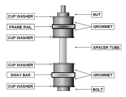
14. Assemble the end links to the Belltech sway bar, as shown in the diagram.
