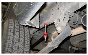
18. Torque the Belltech U-bolts and pivot bushing clamps to 20 ft lbs.
