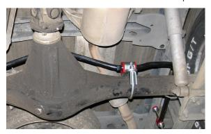
16. Swing the sway bar up and position the ends of the arms as parallel as possible with the holes in frame rails.
