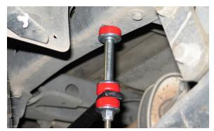
17. Mount the end link assembly to frame and tighten the end link bolt to the point where the spacer tube can still be forced to rotate on the bolt by hand, but the rubber grommets should not be able to rotate by hand.
