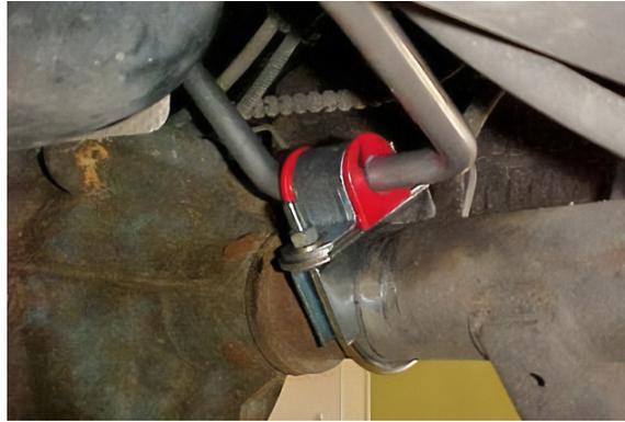
20. Tighten the end link nuts to the point where the spacer tube can still be forced to rotate on the bolt by hand, but the grommets should not be able to rotate by hand. Torque the end link bracket securely to the frame on the passenger side.
