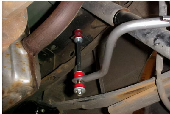
17. On the driver side of the vehicle, locate the 1/2" hole on the lower flange of the frame, in front of the axle. Raise the arms of the sway bar so they are parallel with the frame, the hole on the frame will be above the hole on the sway bar end. Assemble the end link as on the frame and sway bar as shown in the diagram on page four. Place the end link bolt in from above so the bolt head faces up and the nut is at the bottom. Hand tighten but do not torque yet.
