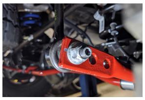
14. Adjust the position of the sway bar so it is centered. Torque the pivot bushing bracket bolts to 41 ft lbs.
