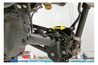
8. Remove the 16mm pivot bushing bracket bolts to detach the sway bar from the vehicle.
