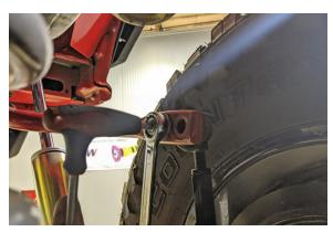
15. Adjust the position of the sway bar so it is centered. Torque the pivot bushing bracket bolts to 46 ft lbs.
