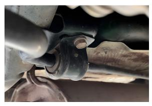
9. Slide the sway bar up and over the exhaust to remove the sway bar from the vehicle.
