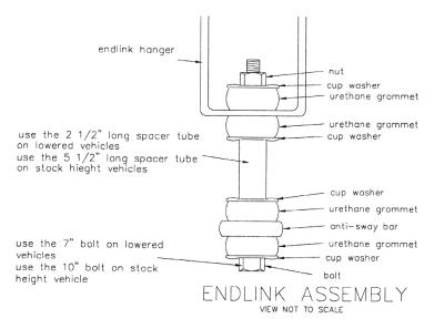
19. Ensure the sway bar is centered directly under the axle. Torque the U-bolts and pivot bushing clamps to 20 ft lbs.
