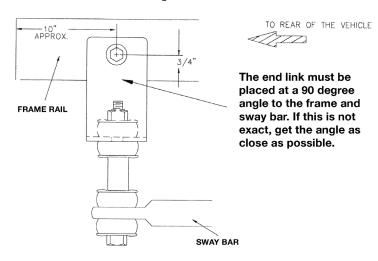
16. Center punch the marks and drill a 3/8" hole through both sides of both frame rails.
