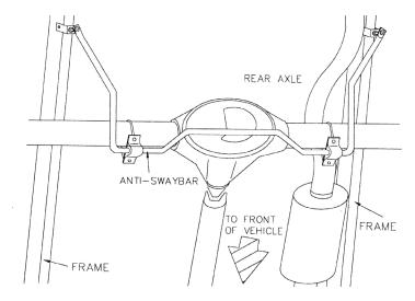
18. Attach the ends of sway bar to the end link hangers as shown in the diagram. Assemble the end links with the 2-1/2" spacer tube and 7" bolt for a lowered ride height or use a 5-1/2" spacer tube and a 10" bolt for a original ride height as shown in the diagram. Tighten the end link nuts to the point where the spacer tube can still be forced to rotate on the bolt by hand, but the grommets should not be able to rotate by hand.
