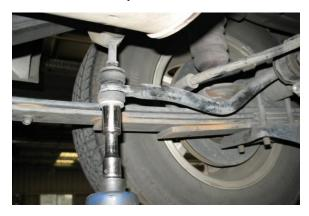
8. Remove the four 18mm U-bolt nuts at the axle clamp to detach the clamps and sway bar assembly from the vehicle.
