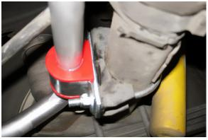
15. The sway bar is positioned vertically behind the axle and the original U-clamp has a small cut out to align it on the axle as shown in the image below. Hand tighten the supplied nuts on the U-bolt for now.
