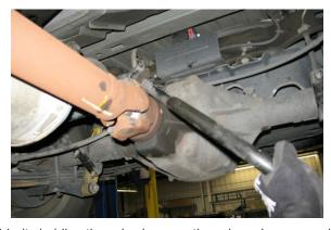
10. Remove the retaining clips from U-bolts holding the axle clamp on the axle and remove axle clamp assembly from the vehicle.
