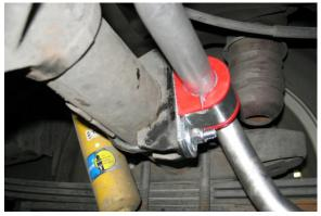
16. Attach the sway bar to the end links using the original hardware; torque to 50 ft lbs.
