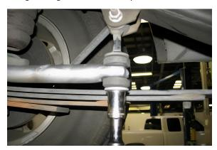
17. Adjust the position of the sway bar so it is vertically behind the axle. Torque the pivot bushing U-bolts to 44 ft lbs.
