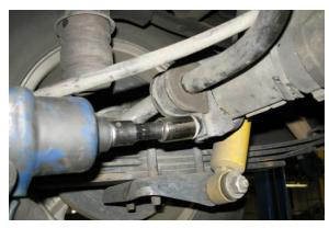
9. Guide the sway bar up and over the driveshaft to remove it from the vehicle.
