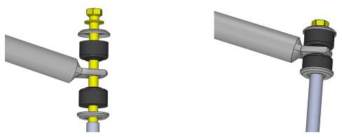
15. The end links must be assembled through the lower control arms and the ends of the Belltech sway bar as shown in the diagram below.
