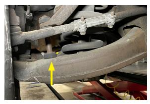
8. Remove the four 10mm pivot bushing bolts to detach the sway bar from the vehicle.
