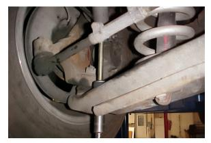
17. Torque the four pivot bushing bracket bolts to 24 ft lbs.
