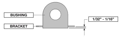
13. Place the Belltech sway bar on the chassis mounts and fasten the pivot bushing brackets with the original bolts. Do not torque yet. Ensure the arms of the sway bar are resting over the tie rods before fastening the hardware.
