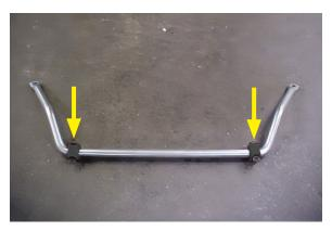
12. Ensure there is 1/32" to 1/16" of the bushing is showing after the bracket is seated. If the bushing is showing more than 1/16", use a sander or a sheet of coarse grit sandpaper to shave it down to the proper height.
