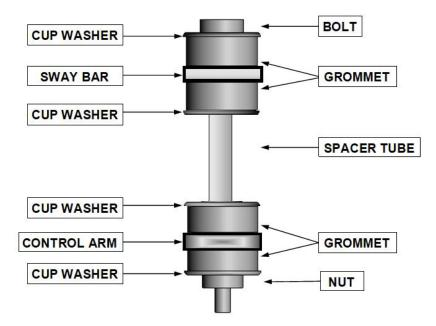
16. Fasten the end link assemblies to lower control arms. Tighten the end link nuts to the point where the spacer tube can still be forced to rotate on the bolt by hand, but the rubber grommets should not be able to rotate by hand.
