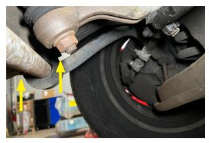
9. With the sway bar removed, clean the mounting surfaces at the chassis and controls arms.
