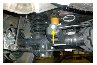
9. Attach the top end of the Belltech track bar bracket to the bolt hole on the original mount. Use the original bolt and tab nut with the supplied tube spacer between the mount. Fasten but do not torque yet.
