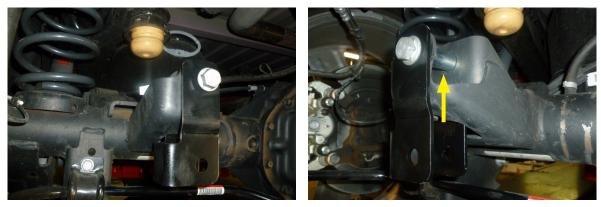
10. Attach the bottom of the track bar bracket up through the support tab and original mount with the supplied 3/8"-16 x 1-1/4" bolt, two 3/8" washers, and Nyloc nut. Torque the 3/8" bolt to 30 ft lbs.
