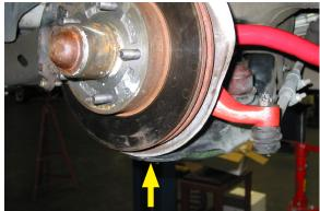
29. If there is severe "toe-out" in the wheel positioning, loosen the two 13mm nuts on the tie rod adjusting sleeves and turn them approximately 2 to 2.5 turns or until wheels appear straight. This will temporarily adjust the toe-in of the vehicle to enable you to drive the vehicle to an alignment shop. Tighten the tie rod clamp bolts and torque to 18 ft lbs.
