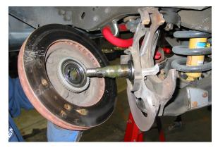
11. Locate the 13mm ABS cable retainer bolt on the upper control arm. Use a ratchet and wrench to remove the nut and bolt. Ensure there is no accidental damage to the cable, retainer, or the mounting hardware. Move the ABS cable out from behind the upper control arm to prevent damage during the dust shield removal.
