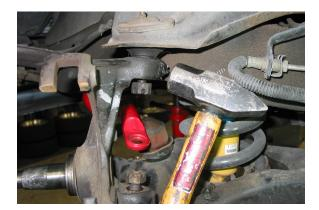
17. Once they are both loose, remove the upper nut and lift the control arm to free the spindle. Now remove the lower nut and slide the spindle off the lower ball joint.
