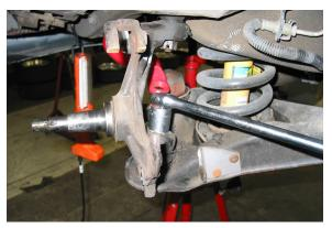
16. Loosen the 22mm upper ball joint nut with the same procedure as the lower, leaving the nut on the threads. Using the hammer method as above, loosen the upper ball joint from its position.
