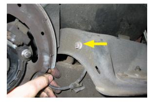
12. Remove the upper and lower 10mm bolts; and the 13mm bolt near the ABS sensor from the face of the cover. DO NOT remove the upper ABS sensor bolt. Detach the cover from the spindle and safely hang it behind the spindle.
