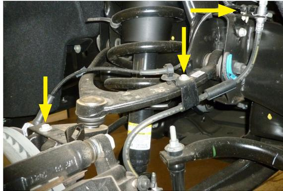
10. Remove the 5mm hex key bolt to detach the wheel speed sensor at the hub bearing
