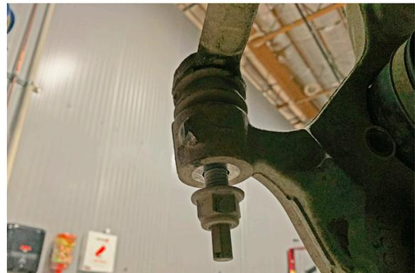
16. Break loose the 18mm upper control arm ball joint nut with. Keep the ball joint nut partially threaded on to the ball joint; doing so keeps the arm from swinging up and helps hold the assembly in place. Use a ball joint removal tool to dislodge the upper ball joint stud from the spindle.
