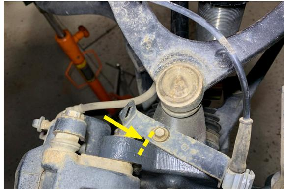
32. Rotate the spindle in both directions to confirm the brake line and ABS line have enough slack. If one or the other is too tight, pull the line through the bracket to give it the proper amount of slack.
