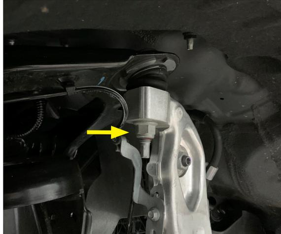
12. Remove the upper ball joint nut with an 18mm wrench. Use the hex stud on the ball joint to prevent the stud from turning while removing the nut. Use a ball joint separator tool to detach the ball joint from the knuckle. Alternatively, you can strike the ball joint boss on the spindle to dislodge the ball joint.
