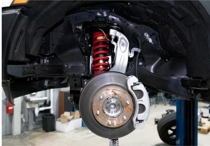
20. Torque the upper ball joint nut to 46 ft lbs.
