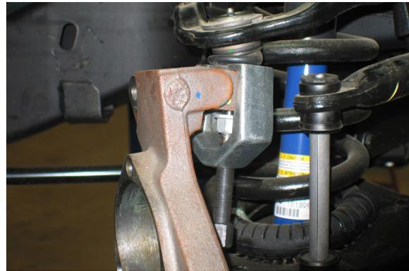
14. Remove the 21mm tie rod end nut and detach the outer tie rod from the steering knuckle using the same ball joint removal tool.
