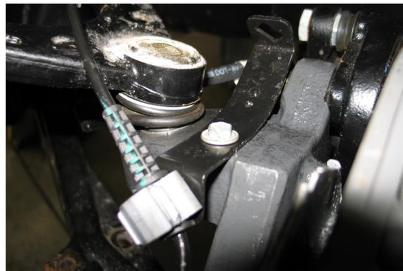
25. Rotate the spindle in both directions to confirm the brake line and ABS line have enough slack. If either is too tight, then you pull it through the bracket to give it the proper amount of slack.
