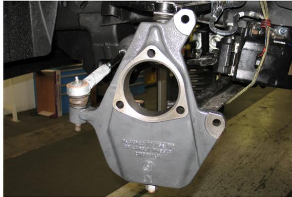
18. Torque the upper ball joint nut to 37 ft lbs.
