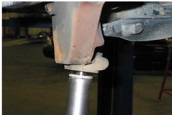
16. Remove the steering knuckle from the vehicle.
