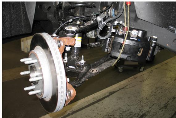
11. Remove the three 15mm bolts on the backside of the hub assembly, detach it from the steering knuckle.
