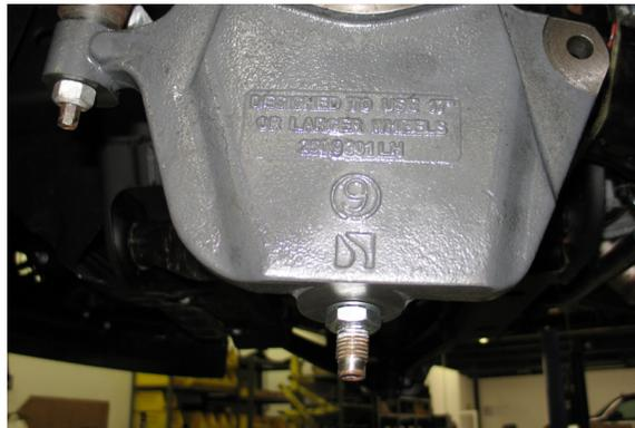
20. Attach the steering tie rod end to the spindle and torque to 44 ft lbs.
