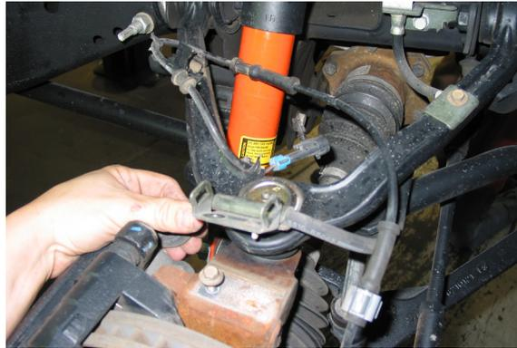
10. Remove the 18mm bolts holding brake caliper assembly from the steering knuckle. With a metal wire or bungee cord attach the caliper to the chassis to prevent damage to the brake line. Next, remove the brake rotor and set aside.
