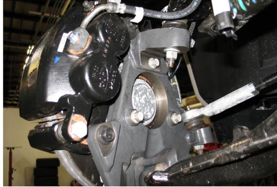
24. Attach the brake line and ABS line brackets, ABS sensor plug on the frame, and the hold down clips in their original locations.
