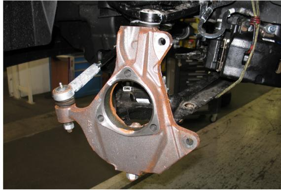
13. With a 18mm socket, break loose the upper ball joint nut but keep the nut partially threaded on the stud to keep the arm from swinging up and to keep it in place while removing the lower ball joint. Using a ball joint separator tool, free the upper ball joint from the steering knuckle.
