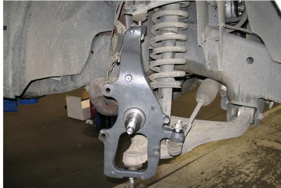
19. Tighten the upper ball joint nut in place and torque to 85 ft lbs.
