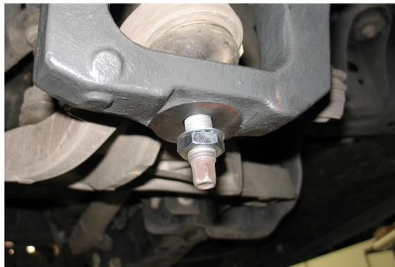
21. Attach the tie-rod end to the spindle, torque the original nut to 111 ft lbs.
