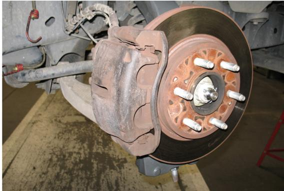
27. Rotate the spindle assembly in both directions to confirm if the brake line and sensor cable have proper clearance. If needed, adjust as necessary.
