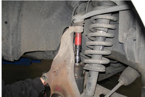
16. Remove the 24mm lower control arm ball joint nut. Use a puller tool to detach the ball joint from the spindle. Alternatively, you can leave the nut on the ball joint and strike the spindle with a hammer to dislodge the ball joint. Do not hit the boot.
