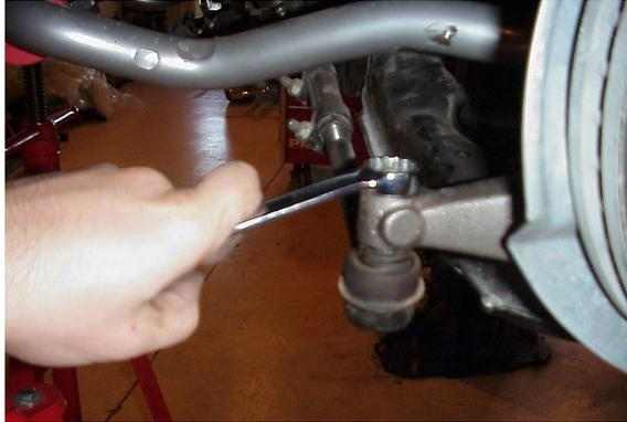
11. Using a hammer, strike the side of the steering arm until the tie-rod end disengage from their tapered bore. Move the tie-rods up and away from the spindles, toward the front of the vehicle.
