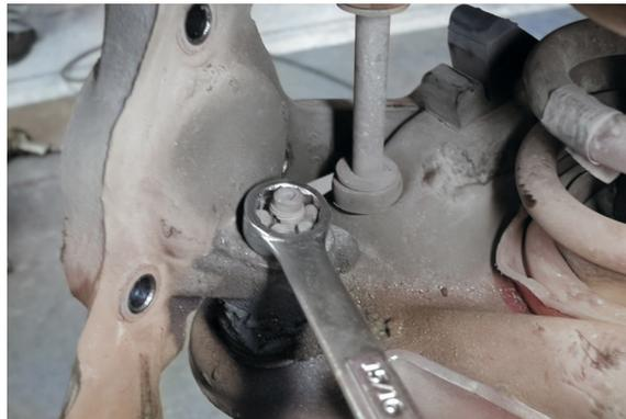
21. Once they are both loose, remove the upper nut and lift the control arm to free the spindle. Now remove the lower nut and slide the spindle off the lower ball joint.
