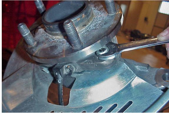
31. From the back of the spindle, loosely thread two of the original hub attachment bolts through the holes in the spindle into the threaded holes of hub flange. Ensure the hub diameter SQUARELY aligns into the central bore of the lowering spindle.
