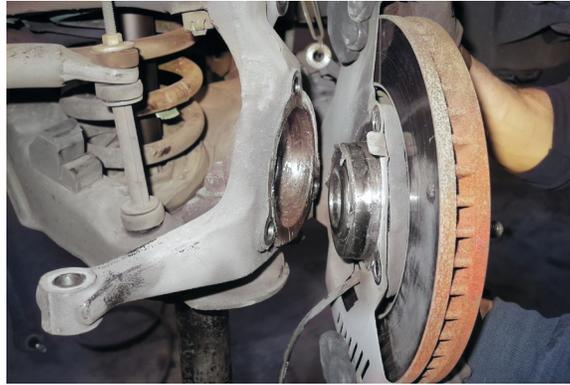
17. Place a floor jack under the lower control arm and lift until a slight compression of the suspension is achieved. Turn the spindle to access the ball joints without interference.
