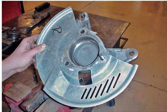
28. Place a thin coating of chassis grease or anti-seize compound on the diameter of the hub assembly that mates with the central bore of the lowering spindle.
