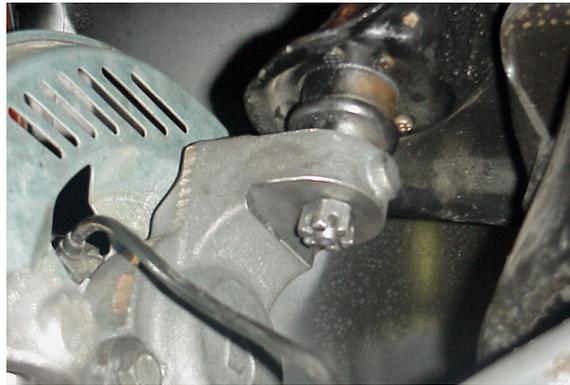
35. Place the brake rotor over the wheel studs and onto the hub assembly to its original position. Mount the brake caliper assembly over the brake rotor while aligning the mounting bracket with the mounting holes in the spindle. Ensure not to twist or stretch the brake hose and ensure the brake pads fit properly over the brake rotor. Torque the two caliper bolts to 133 ft lbs.
