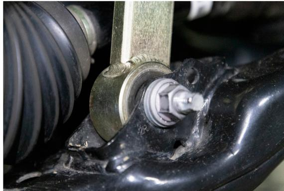
30. Attach the lower bracket to the spindle and lower ball joint. Torque the lower ball joint nut to 103 ft lbs. and the lower bracket bolts to 118 ft lbs.
