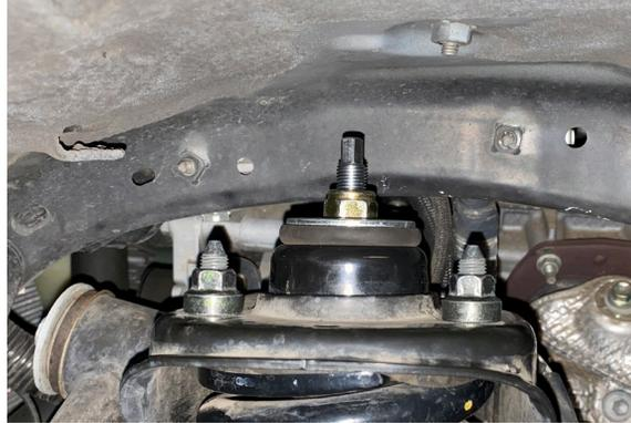
29. Attach the lower coilover mount to the lower control arm using the original nut and bolt. Once the suspension is stabilized, torque 61 ft lbs.
