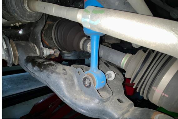
13. Mark the alignment of the camber and caster adjustment bolts securing the lower control arm to the frame. This will help keep the alignment close to the original settings when installing the control arms.
