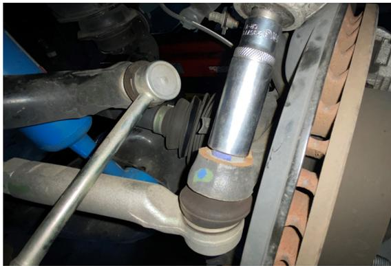
11. Remove the 24mm lower ball joint nut, the two 19mm lower bracket bolts, and detach the lower bracket from the spindle. This will allow the spindle assembly to be moved to the side for clearance. Use a strap or rope to tie the spindle assembly to the chassis.
