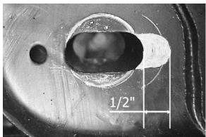
3. Use a die grinder with a carbide cutting tip to carefully elongate the slat towards the center of the vehicle. Do no elongate beyond the 1/2" outlined as this will allow the control arm to contact the frame.
