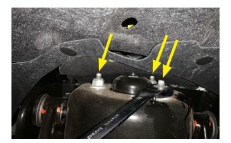
21. Attach the lower strut mount to the lower control arm using the supplied flanged bolts and Nyloc nuts. Torque the supplied nuts to 66 ft lbs.
