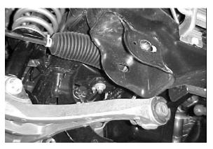
2. Scribe a 1/2" line inward from the edge of the factory alignment slot in the chassis. This must be done to all four slots on each side of the vehicle.
