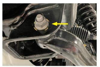
10. Working on one side at a time, use a 21mm and 27mm wrench to remove the cross member nuts and bolts that connect the lower control arm and frame.
