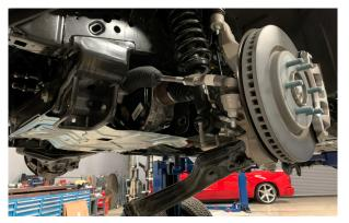
13. Remove the three top mount 18mm nuts that secure the top of the strut to the chassis.
