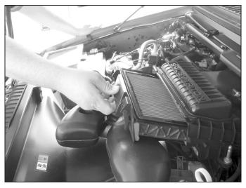
3. Slide the tray with the AIRAID® air filter back into the airbox.
