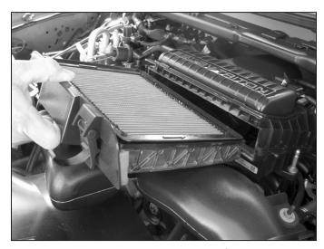
2. It is very important to place the AIRAID  $\!^{\text{@}}$  air filter in tray with the orientation arrows facing the airbox.
