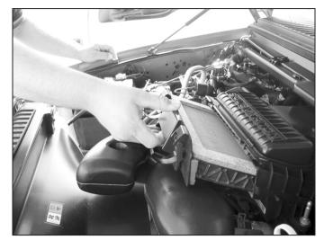
1. Unfasten clamps and slide the tray out from airbox, remove the stock air filter. Wipe away dirt and debris from the tray and airbox.
