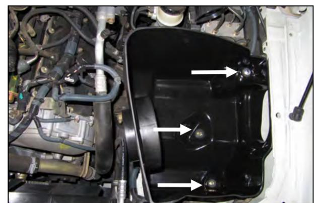
6. Set the CAB assembly inside the engine compartment, align the bolt holes, and secure using the OEM hardware.
