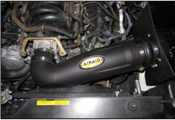
10. Install the Airaid Intake Tube into the Hump Hose first, and then press the reducer onto the throttle body. Adjust for fit, and tighten all four Hose Clamps.
