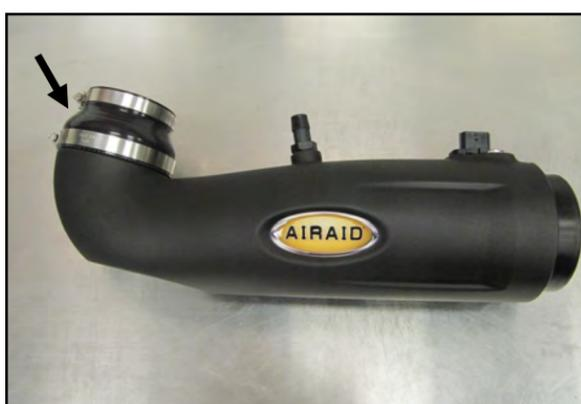
8. Slip the Silicone Reducer (#5) onto the Intake Tube as shown. Slide the #64 Clamp (#19) onto the Reducer first, followed by the #48 Clamp (#18). Leave the Clamps loose for now.
