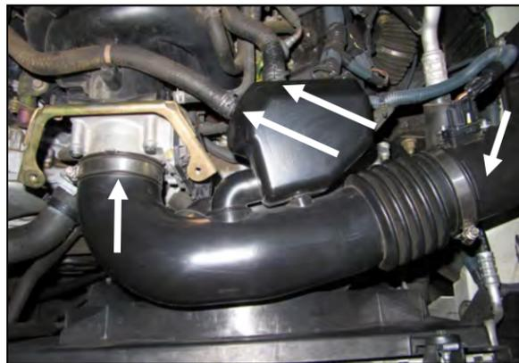
2. A.) Using a pair of pliers, compress the spring clamps on the PCV breathers and then slide back. Disconnect the breathers from the factory intake
