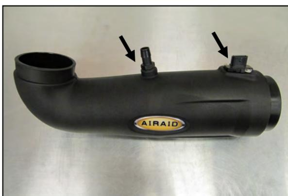
7. Install the threaded 5/8" Barbed Fitting (#15) into the Airaid Intake Tube (#2). Transfer the Mass Air Flow sensor from the factory airbox, into the Airaid Intake Tube and secure using the two 8-32 Button Head Screws. Do not attempt to reuse the factory screws. Apply the Airaid Decal to the Tube as shown.
