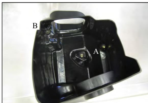
5. Transfer the airbox mounting grommets and hardware from step 3. into the Cold Air Box. A.) Insert the large mounting grommets and bolts from the inner fender into the bottom of the CAB. B.) Remove the small grommet and steel sleeve from the top of the airbox and install it remaining hole in the CAB.
