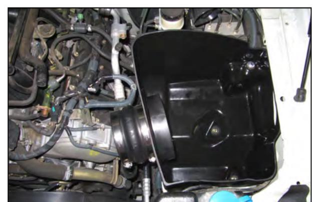
9. Slide the Hump Hose (#6) and #72 Hose Clamps (#20) onto the Filter Adapter. Leave the clamps loose for now.
