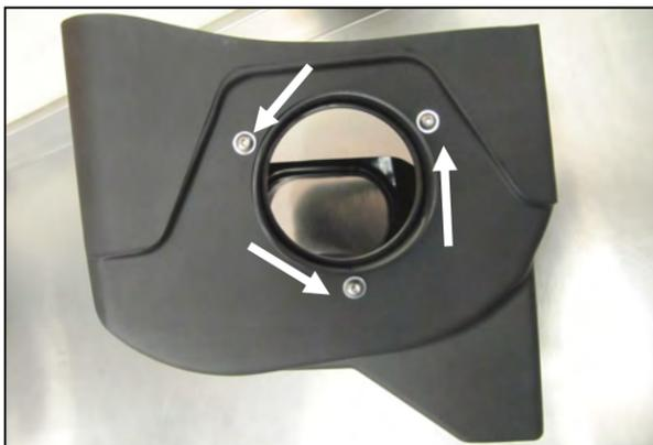
4. Install the Filter Adapter (#4) onto the Cold Air Box (#3), or CAB, as shown using three 1/4-20 Button Head Bolts (#9), and 1/4" Flat Washers (#12). Refer to the line drawing above for details.
