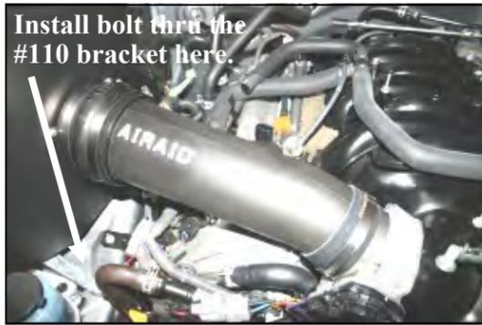
Install bolt thru the #110 bracket here.
