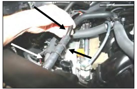
**12.** Install the 1/2" breather hose (#23) onto the nipple on the Airaid tube. Slide the 1/2" barbed coupler (#21) into the installed breather hose, and secure both ends with the supplied speed clamps (#22).
