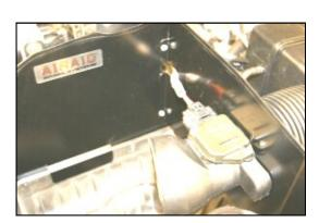
7. Install the MAF sensor into the MAF adapter (#4) and tighten down using two  $8-32 \times 1/2$ " button head bolts (#22). Do Not Use The Factory Screws!
