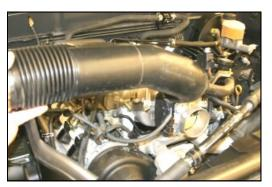
12. Remove the factory intake tube.
