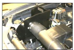
5. Slide the MAF adapter into the factory tube, and at the same time slip the CAD onto the top of the factory airbox base, adjust for fit and relatch the 3 factory clips. Tighten the hose clamp on the factory intake tube. Reinstall the shroud
