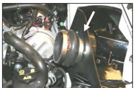
10. Install the hump hose (#5) on the filter adapter (#6), with two #72 hose clamps (#13). Tighten only the clamp next to the CAD.
