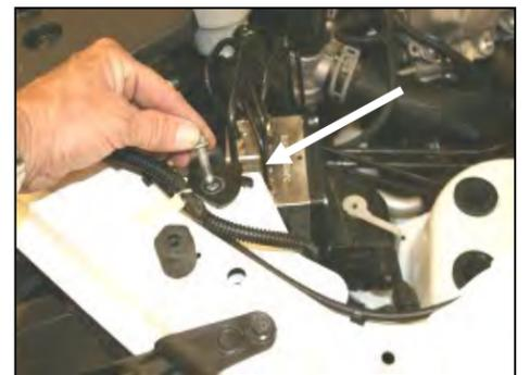
6. With a 10mm socket, remove and save the bolt from the anti-lock brake bracket. It will be re-installed later in step #8.
