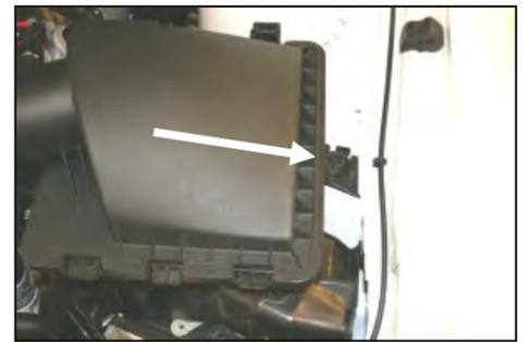
3. With a 10mm socket, remove the bolt holding the factory airbox to the fender and save the bolt. It will be reused
