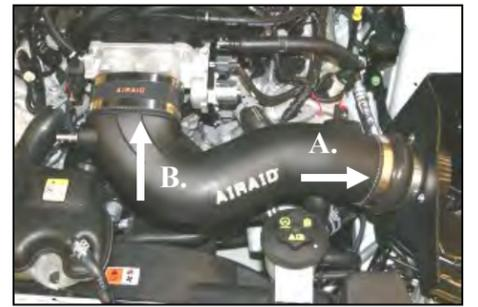
15. A.) Install the tube into the hump hose. B.) Now slide the oval coupler onto the throttle body. Tighten the remaining two hose clamps, and re-connect the mass air sensor, from step #2.
