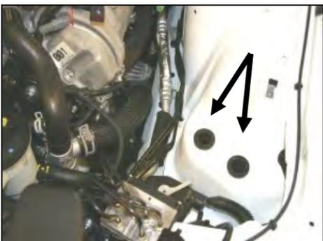
4. Remove the complete factory intake. Use caution to retain the factory grommets in the inner fender.
