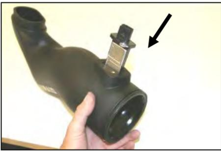
13. Align the two slots in the tubes, and install the factory mass air sensor removed from step #5. Make sure the screw holes line up, then install the two supplied button head screws. (#12). **DO NOT USE THE FACTORY SCREWS!!**
