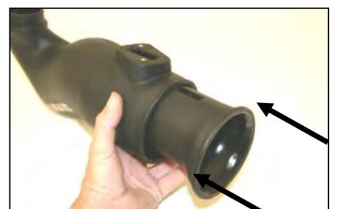
12. Install the Modular Venturi Tube (MVT) (#3) into the Airaid Intake Tube (#2) as shown. (SEE #22 BELOW!!)
