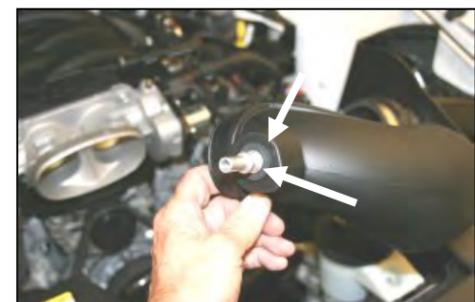
11. Install the supplied grommet (#14) and aluminum fitting (#17) into the Airaid intake tube as shown.
