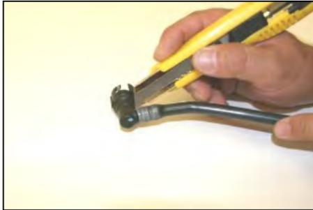
17. **VERY CAREFULLY!** Using a razor blade, cut the plastic tube off both of the factory breather hose ends as shown.
