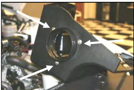
7. Install the air filter adapter (#6) into the Cool Air Dam (#7) as shown, using 3 button head screws (#10) and 1/4" flat washers (#11).
