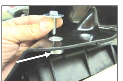
9. Slide the Aluminum Spacer (#15) underneath the CAD and into the hole as shown. Secure the CAD to the inner fender using the OEM bolt from step #3 and the supplied 1/4" Fender Washer (#16).
