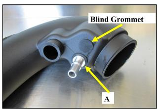
4. Install the Grommets and Fittings into the Airaid intake 5. Using the supplied Torx driver, remove the MAF sentube A) All models will require the use of the 5/8" Fitting sor from the factory airbox and create the Tube assem-(#19) and the 5/8"Grommet (#20). **B)** Automatic trans- bly. mission equipped vehicles will also use the 3/8" Fitting (#18) and 3/8" Grommet (#21). Manual transmission vehicles will not need the 3/8" components and will use the Blind Grommet(#22).
