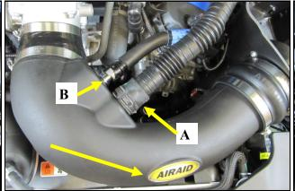
11. Install the Airaid Intake Tube into the couplers as 12. A) Install the Airaid Premium Filter onto the filter shown, and tighten all Hose Clamps. A) Reconnect the adapter and tighten the hose clamp. B) re install the Reso-Resonator tube to the Airaid Intake using the OEM nator tubing into the factory Stand off. clamp. B) Reconnect the breather line/lines to the Aluminum Fittings depending on your application. Apply the Airaid Decal onto the Tube as shown.
