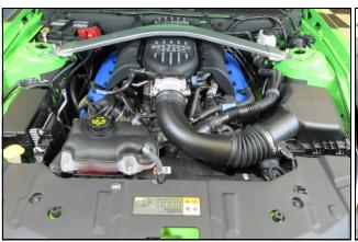
1. Disconnect The Negative Battery Terminal. Additional Installation Note: This Intake system can also be installed on a Mustang GT 5.0L with the Boss intake manifold conversion and contains the fitting required to connect the brake aspirator line for AT equipped vehicles.
