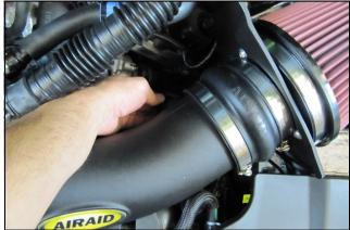
located in the lower back side of the intake. Slide the locking tab back into the connector.
