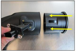
A) Slide the Modular Venturi Tube (#3) into the Airaid intake tube (#2) making sure to align the two slots for the MAF sensor. B) Install the MAF sensor into the intake tube using two provided 8-32x3/8" screws (#12).
