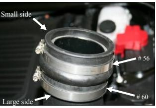
the CAB tube. Loosely install the #56 Hose Clamp (#10) on the small side of the Hump Hose, and the #60 Hose Clamp (#11) on the Large side. ( B) Slide the Hump Hose and Clamps downward on the tube, creating a compact assembly as shown.
