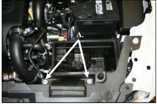
**4. A.)** Using an 8mm socket, remove the two factory air **5.** Remove the factory air box assembly from the vehicle. box bolts and set aside. The will be reused in step 11. B.) Remove the factory air filter element.
