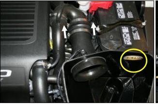
tory Air box and secure using the factory hardware from adapter and tighten the clamp. step 4. B.) Slide the coupler and clamps onto 90 deg. Elbow pipe and tighten the clamps. C.) Reconnect the Air Temperature Sensor. Apply the Airaid Decal inside of the Airbox as shown.
