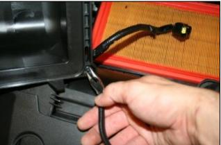
the fins of the wiring harness anchor and pull it out of the air box lid.
