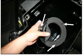
**6.** Prepare the Filter Adapter (#3) for installation by positioning the Adapter Gasket (#12) on the mounting side and lining up the holes.
