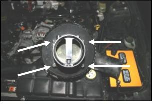
**5.** Remove the four bolts that hold the **MAF** housing to the factory air filter canister. The bolts will not be reused, but the **MAF** housing will be used in the next
