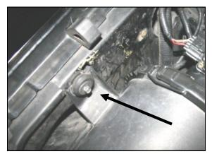
**3.** Remove the bolt that holds the factory air filter canister to the inner fender. Next remove the factory air intake tube from the throttlebody, and then the **MAF** housing. Now with a twisting motion remove the factory air filter canister from the vehicle.
