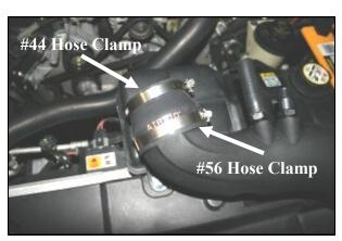
**8.** Install the reducer coupler (#4) onto the throttle-body end of the Airaid Intake Tube using the #56 hose clamp (#14) on the tube end, and the #44 hose clamp (#13) on the small end. Tighten *only* the large #56 clamp at this time.
