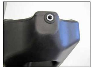
8. Install the provided grommet and spacer into the AIRAID<sup>®</sup> air filter housing as shown.
