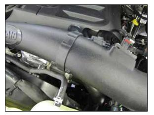
19. Secure the mass air sensor wiring clip to the intake tube.
