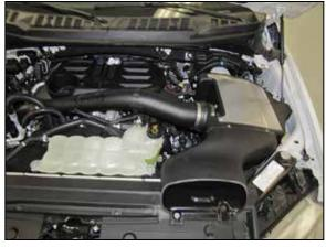
**21. Double check your work!** Make sure there is no foreign material in the intake path. Make sure all clamps, hoses, bolts, and screws are tight. Double check the hood clearance! **Reconnect the negative battery cable!**
