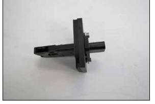
13. Install the provided gasket onto the mass air sensor adapter. Remove the mass air sensor from the factory housing and then install it into the AIRAID<sup>®</sup> adapter and secure with the provided hardware.
