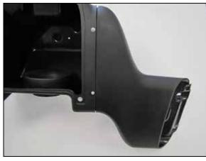
10. Install the AIRAID<sup>®</sup> fresh air intake duct into the air filter housing and secure with the provided hardware.
