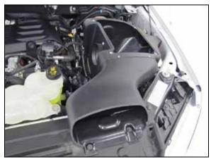
11. Install the AIRAID<sup>®</sup> air filter housing assembly into the vehicle and secure with the provided hardware.
