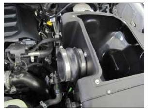
12. Install the provided hump coupler onto the filter adapter and secure with the provided hardware.
