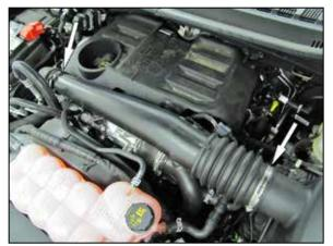
4. Loosen the two hose clamps that secure the factory intake tube and then remove the tube from the vehicle.
