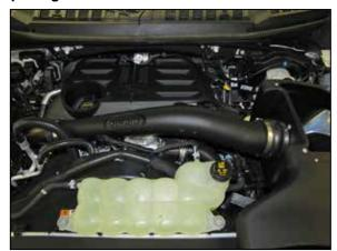
15. Install the AIRAID<sup>®</sup> intake tube into the factory turbo inlet coupler and the coupler at the filter adapter, adjust the tube for best fit and then secure with the provided hose clamps.
