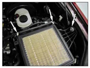
7. Disconnect the mass air sensor wiring harness from the lower air filter housing. Remove the bolt that secures the lower air filter housing to the inner fender and then remove the lower housing from the vehicle.
