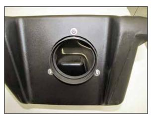
9. Install the provided filter adapter into the AIRAID<sup>®</sup> air filter housing and secure with the provided hardware as shown.
