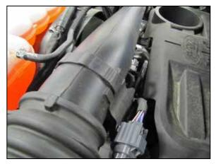
3. Disconnect the mass air wiring harness clip from the intake tube.
