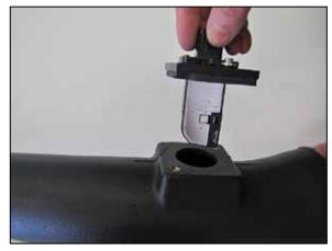
14. Install the mass air sensor adapter into the AIRAID intake tube and secure with the provided hardware.
