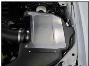
17. Install the AIRAID<sup>®</sup> air filter onto the adapter and secure with the provided hose clamp and then
