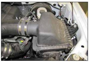
14. Reinstall the upper air filter housing onto the lower housing and into the coupler on the intake tube. Secure the housing to the lower housing with the factory clips and to the intake tube with the provided hose clamp.
