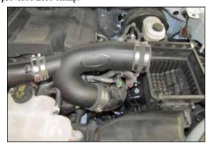
12. Install the AIRAID intake tube onto the turbo inlet tubes and secure with the provided hose clamps.
