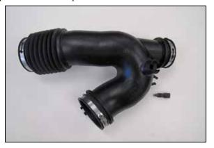
9. Remove the inlet air temperature sensor from the factory intake tube and remove the O-Ring from the sensor.
