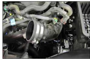
7. Install the provided coupler hose (5-400) onto the driver's side turbo inlet tube and secure with the provided hose clamp.
