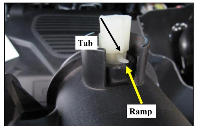
**9.** Remove the Air Temperature Sensor from the factory air box. Gently push back on the sensor so the locking tab will clear the ramp and rotate the sensor 1/4 turn counter clockwise. The sensor is now free and can be pulled out.
