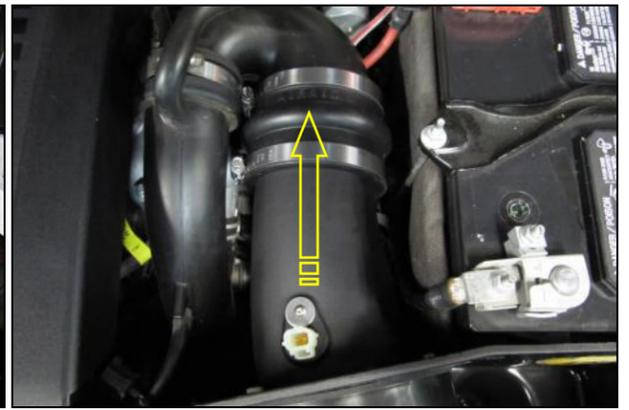
12. Slide the coupler and clamps onto 90 deg. Elbow pipe and tighten the clamps.
