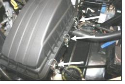
2. Unlatch the three metal clips that hold the airbox lid
