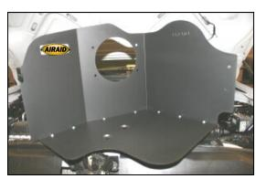
9. Assemble the two Cool Air Dam panels (#2 and #3) as shown, using seven 6-32 screws (#10), #6 washers (#11), and keps nuts (#12). Tighten securely. Apply the Airaid Foil Decal onto the Panel as shown.
