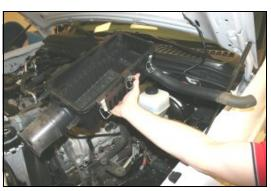
4. Remove the base assembly by pulling it up out of the mounting grommets. Using the supplied torx bit (#14), 1/4" socket, ratchet and extension remove the two screws holding the factory mass air sensor in place, and remove the mass air sensor from the air cleaner lid.
