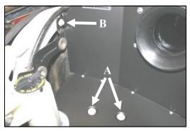
11. A.) Align the two panel holes with the air cleaner base support holes on the vehicle.
