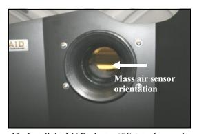
**10.** Install the MAF adapter (#4) into the panel, using four 1/4-20 button head bolts (#6), and 1/4" washers (#7). Be sure to orient the tube with the mass air sensor to the rear of the vehicle. Using a 5/32" allen wrench, tighten the 4 bolts securely.
