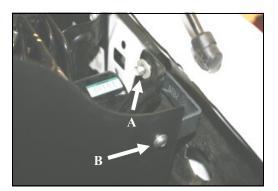
12. A.) Slide the L-bracket under the anti lock braking system bracket, and re-install the bolt removed in step #8.
