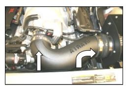
**14.** Install the Airaid Intake Tube into the hump hose first, and then onto the throttle body, making sure it is flush against the throttle body, adjust for fit, now tighten all of the hose clamps.
