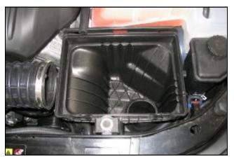
**3.** Remove the factory air box lid and flat panel filter. (*Note: Retain the factory air box base.*)
