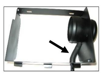
**4.** Install the supplied ½" hose on the Airaid **CAD** nipple. Assemble Airaid **CAD** panels using supplied hardware. Install supplied ½" nylon union through the panel hole into the ½" hose.
