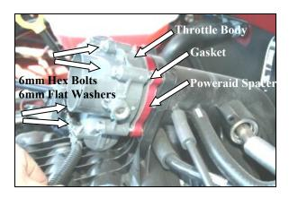
**4.** Install the Poweraid Spacer (#1) with the bore extending into the intake manifold. Install the Gasket (#2) between the Poweraid Spacer and the throttle body. Install four 6mm x 50mm hex bolts (#3) and 6mm flat washers (#4) through the throttle body, Poweraid Spacer, Gasket, and into the intake manifold. Using a 10mm socket, tighten all four throttle body bolts evenly, to the manufacturer's specifications. **Do Not Over Tighten The Bolts!**
