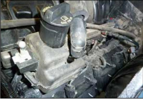
7. Disconnect the crank case vent hose from the valve cover port.
