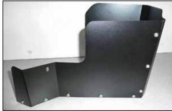
12. Some vehicles may have an AC line obstructing installation. Choose the appropriate heat shield wall for the AC line configuration and attach to the heat shield as shown using the provided hardware.
