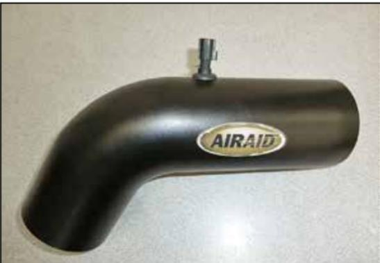
23. Remove the inlet air temperature sensor from the factory tube and install it into the grommet installed into the AIRAID intake tube as shown.
