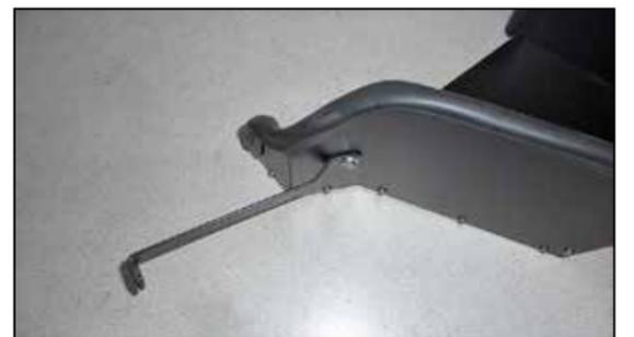
17. Install the heat shield mounting bracket (083103-1A) onto the heat shield using the provided hardware.
