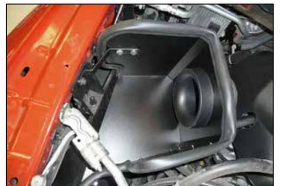
20. Install the heat shield assembly into the vehicle and secure with the bolts removed in steps #18 and #19. Do not completely tighten at this time.
