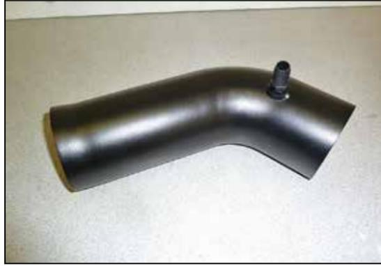
24. Install the 1/4npt vent fitting into the AIRAID intake tube as shown.
