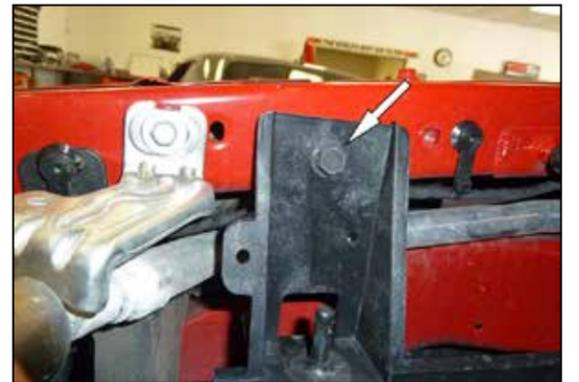
18. Remove the front air box mounting bracket bolt shown.
