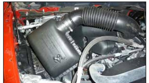
5. Disconnect the factory intake hose from the throttle body, then lift up the air box assembly and then remove it from the vehicle.
