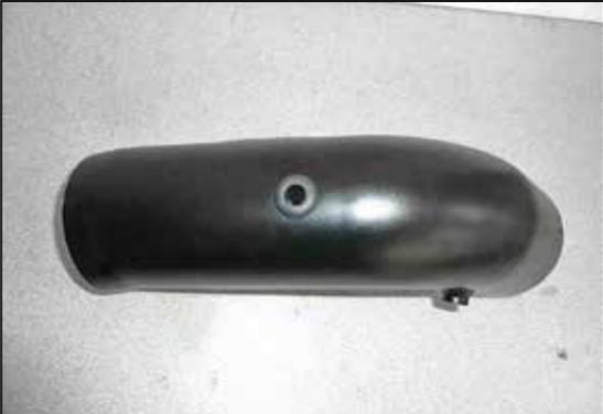
22. Install the provided grommet into the AIRAID intake tube as shown.
