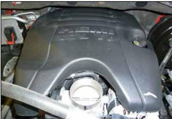
11. Reinstall the engine cover onto the mounting studs and route the crank case vent hose through the opening.
