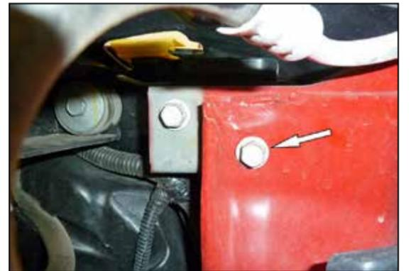
19. Remove the front fender mounting bolt shown.
