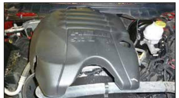
6. Lift up the engine cover to dislodge it from the mounting posts and then remove it from the vehicle.
