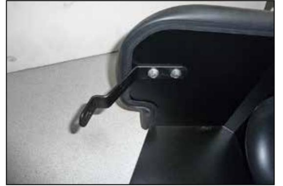
16. Install the heat shield mounting bracket (083127) onto the heat shield using the provided hardware.
