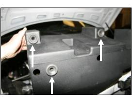
**8.** Install the factory grommets removed in step #3 into the bottom of the **CAB** at the locations shown here.
