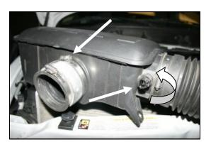
**5. 2002-07 Models** Loosen the factory hose clamp on the coupler and remove the coupler assembly from the resonator. **2003-12 Models** Rotate the air temp sensor counterclockwise and remove it from the resonator. These parts will be reinstalled on the Airaid intake tube in step #12.
