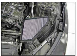
9. On AIRAID Jr. kits **ONLY**, remove the air filter housing lid and replace the stock air filter with the provided AIRAID filter, reinstall the lid and secure with the factory hardware.
