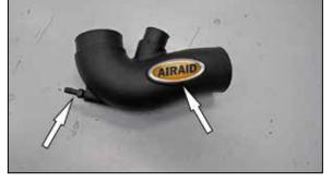
10. Install the AIRAID decal onto the intake tube. Install the provided 1/4npt into the intake tube.
