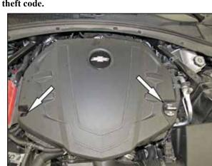
2. Remove the oil cap and bolt that secure the engine cover and then remove the engine cover from the vehicle.
