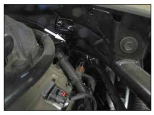
7. Remove the bolt that secures the sound tube to the firewall and then rotate the tube clockwise to remove the complete sound tube assembly.
