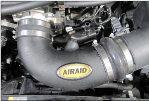
13. Insert the Intake Tube into the coupler first, then into the Hump Hose. Tighten all four clamps at this time.
